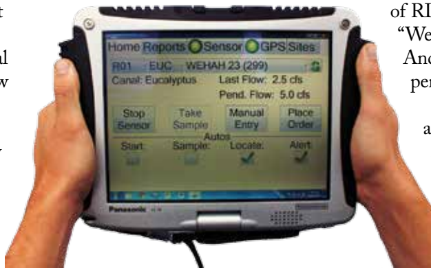
RemoteTracker user interface on a Panasonic Toughbook CF-19. The last flow measurement and any pending flows (i.e., orders) for a site are shown on the home tab. The CF-19 is one of the only tablet PCs that comes with a Class 1 Bluetooth radio, which enables long-range communications (300 feet) between the tablet PC and the wireless water velocity sensor.
